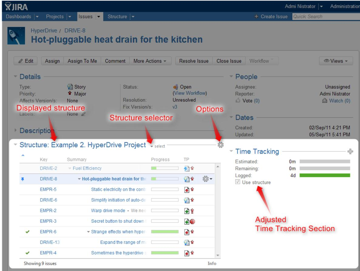
Structure section name includes the name of the currently selected structure.
