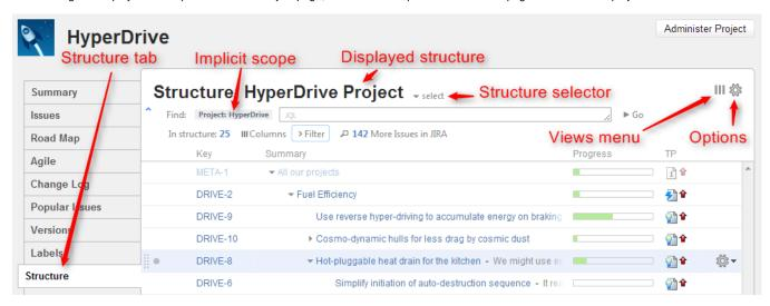
The selected Project (or Component / Version) defines the **scope** of the current structure view - which is used to filter the structure (see details below). For the sake of clarity, we describe the functionality of the structure on the Project page tab; it works in the same way on the Component page tab and Version page tab.
