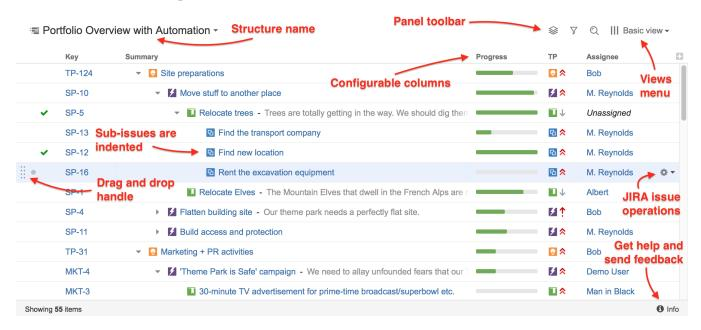
Structure widget is a grid with adjustable columns that displays the issues as a hierarchical list. Structure widget is displayed on the Structure Board, Issue Page and in other places in JIRA.
