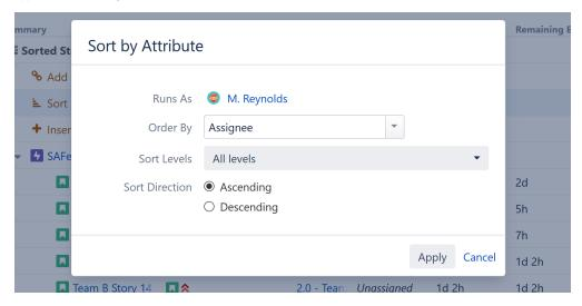
Sort generators can be applied to all levels, the current level only, or to a custom level range.
